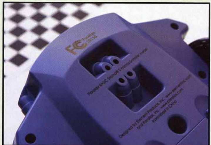
FIGURE 2. The line follower sensor on the bottom of the Scribbler.
